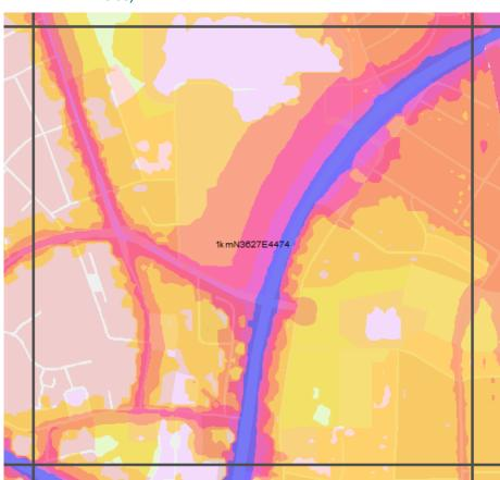
*Figure 3.3: Result of overlaying reference grid cells with noise contour maps (in this case, road noise)*
