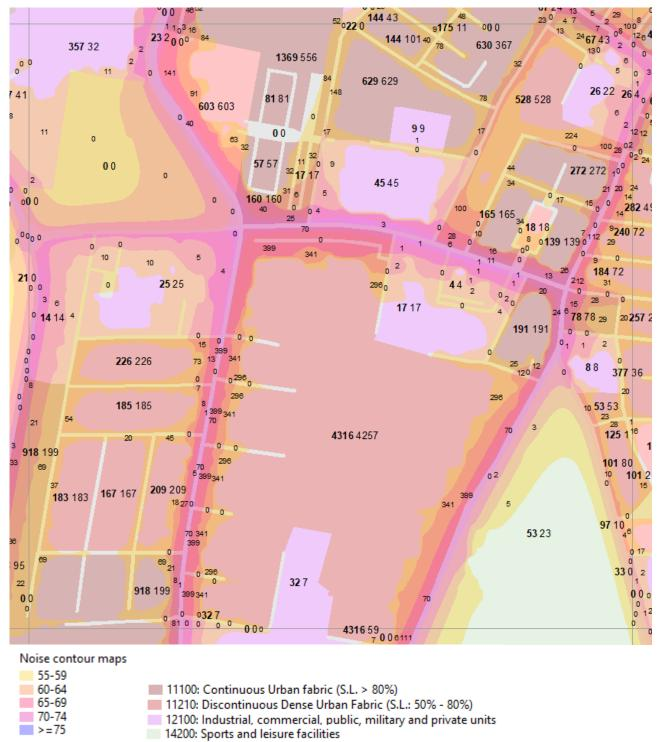
Figure 3.4: Result of calculation of the population per noise contour band area
