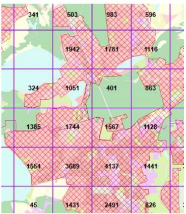
If only one residential polygon of CLC exists in the grid cell all the population is assigned to this polygon. When several residential polygons exists in the grid cell the population is assigned to the residential areas based on area surface.
