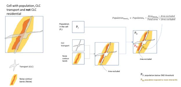
In this case, the grid layer will be overlayed with the noise contour maps. This overlay will enable the calculation of the area of each noise band and assign the number of people exposed according to the percentage of this area in the grid. It is considered that the higher noise bands (> 75dB for L<sub>den</sub> or > 70
