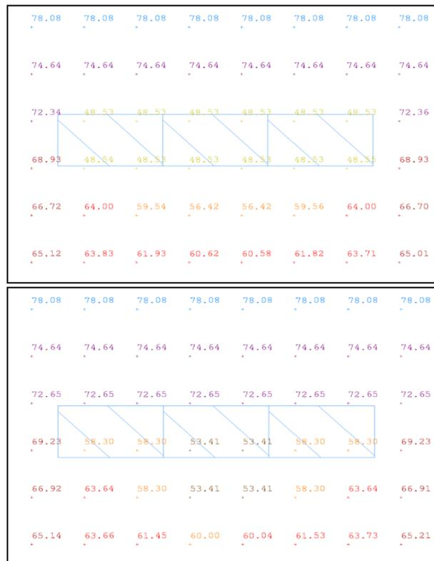
**Figure 5:** Example of how the position of the building polygon with respect to the grid spacing may significantly affect the noise level calculated at the quietest grid point outside the building
