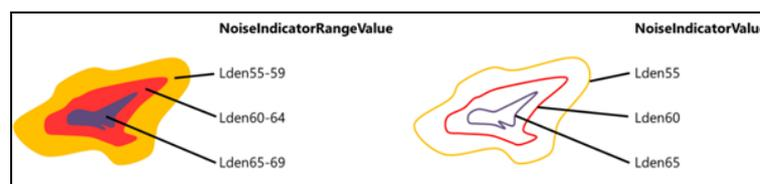
**Figure 2:** Assigning noise level information to noise contours with area or line geometry
