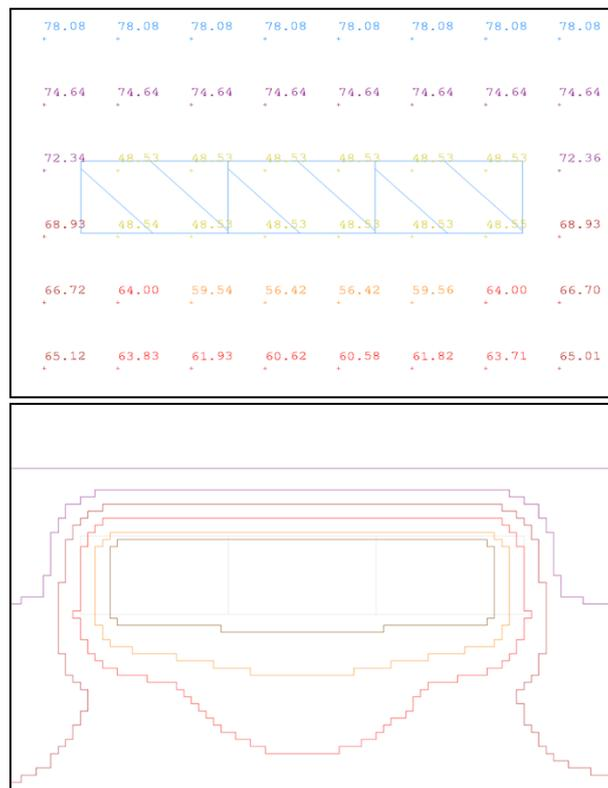
**Figure 7:** Grid with quiet points inside building results in 5 dB contours in front of building which is not realistic
