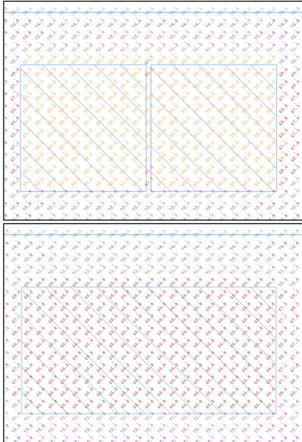
**Figure 6:** Example of how the presence of small gaps between buildings may generate quiet results, but only if they align with the grid receiver points
