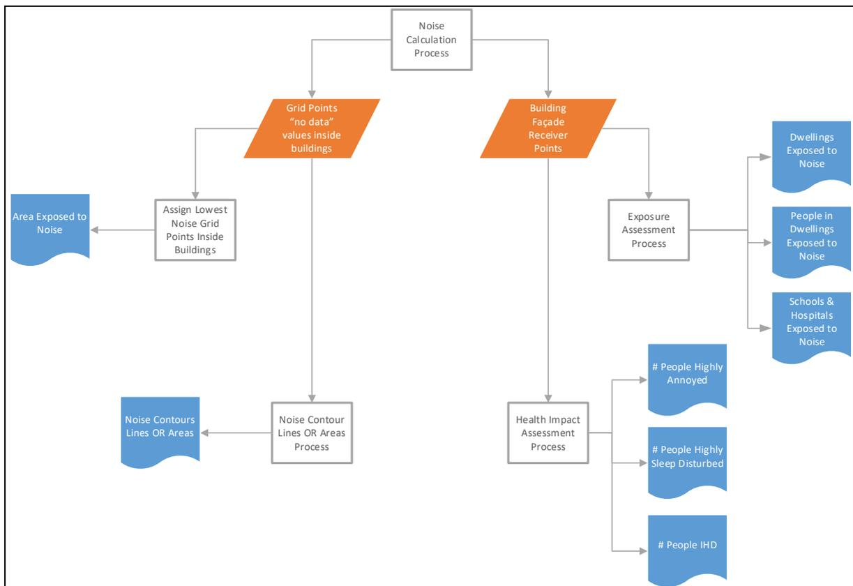
**Figure 10:** Example workflow from noise calculation results to reporting datasets for EEA Reportnet 3 DF4\_8 and DF7\_10
