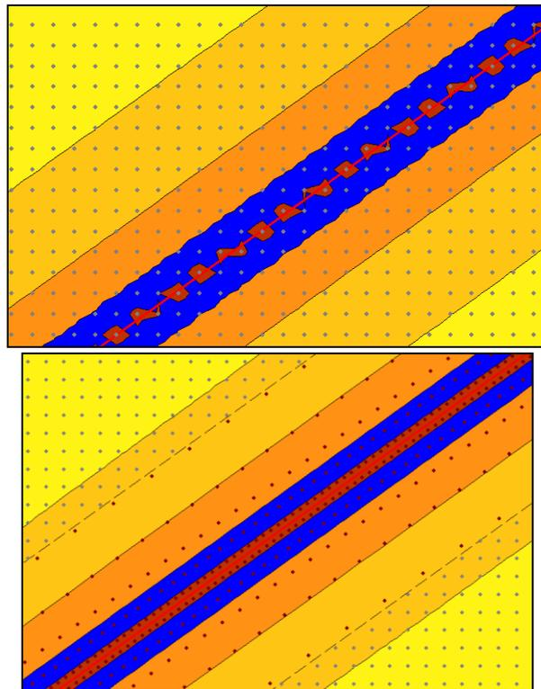
**Figure 4:** Contours created with a regular grid (left) compared to contours with an irregular grid parallel to a noise source (right)
