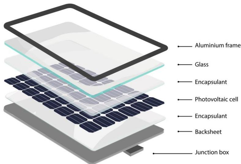
Figure 7.1. Illustration of a photovoltaic panel.
