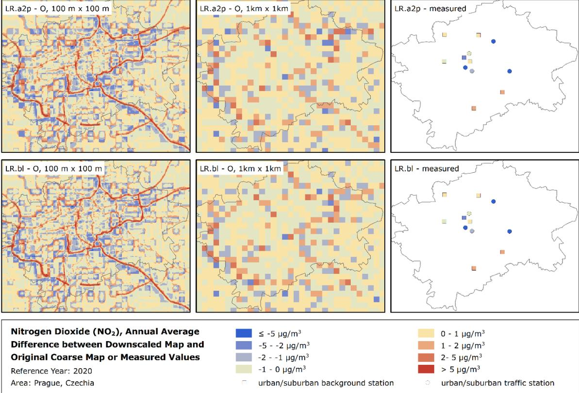
Map 3.1 presents the final fine resolution map of NO<sub>2</sub> annual average 2020 for Prague, as created by the reference downscaling method (LR.a2p), i.e. the linear regression and area-to-point kriging on its residuals. In the map, one can see the main roads in Prague with elevated NO<sub>2</sub> concentrations.
