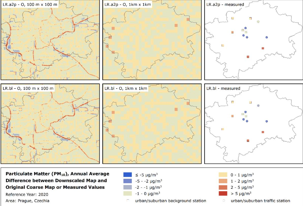
Map 3.2 shows the final fine resolution map of PM<sub>10</sub> annual average 2020 for Prague, as created by the reference downscaling method (LR.a2p), i.e. the linear regression and area-to-point kriging on its residuals.
