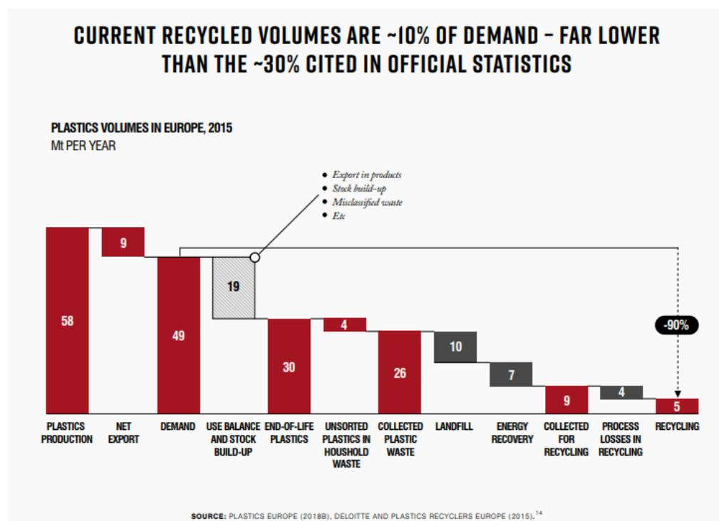
Figure 4.1 Scheme of loss of plastics during plastic waste collection and processing in 2015. (Material Economics 2018)
