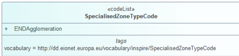
Figure 25. Code list SpecialisedZoneTypeCode applicable to data model for agglomerations (DF1_5)
