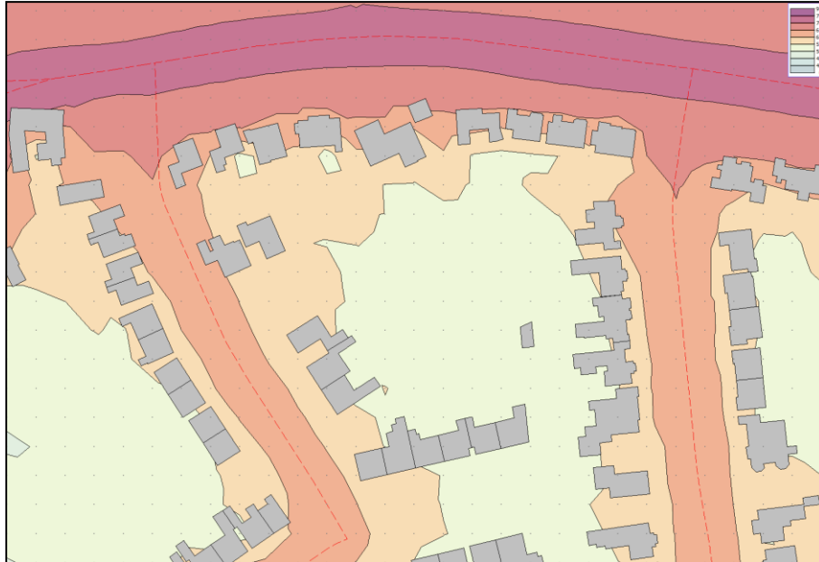
Figure A2.9 Example of noise level contour polygons generated using recommended methodology
