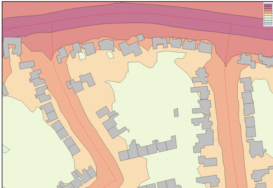
Figure A2.9 Example of noise level contour polygons generated using recommended methodology
