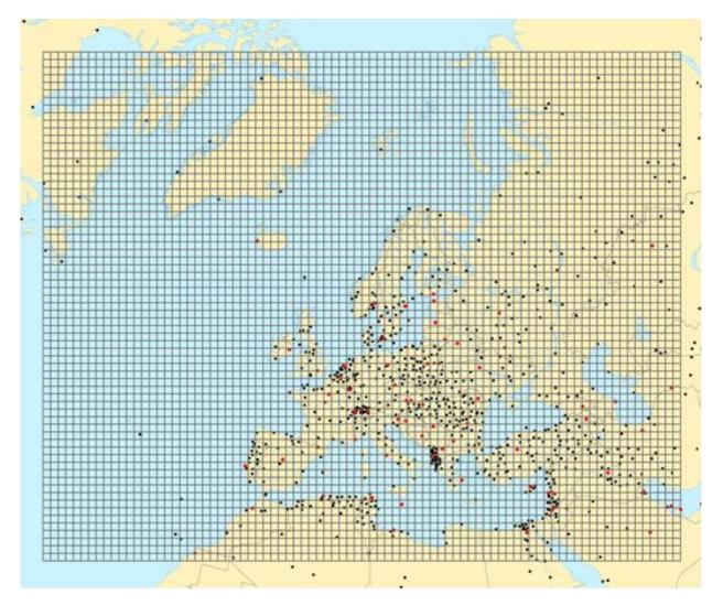
The above map above illustrates a sample of the 100 km ETRS89-LAEA grid. This sample grid covers the area from 0 meters East, 700000 meters North to 6700000 meters East and 9100000 meters North.
